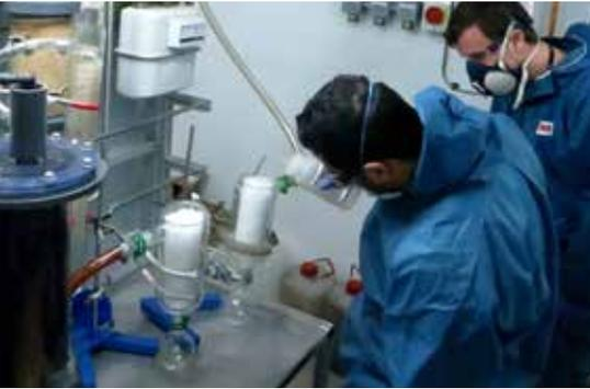
A thermal conversion process known as pyrolysis, which heats material in a reactor vessel containing an oxygen-free atmosphere, can be used to process plastic waste into fuel gas, oils and solid residue (char).
